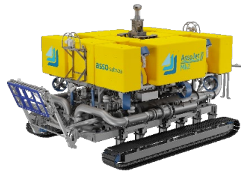
AssoJet III Mk2 Jetting Vehicle (1.56 MW)
