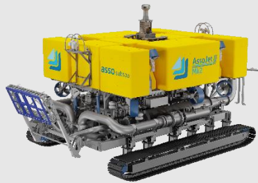
AssoJet III Mk2 Jetting Vehicle (1.56 MW)
